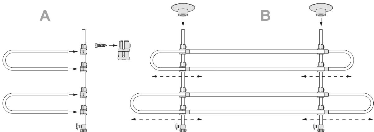
**C)** Screw the Allen screws into the bases of the uprights until they protrude 2 cm. Now slide the rubber foot over the Allen screw.
