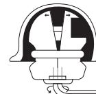
*Fig. 3) Insert the plug-in cylinder lock into the ball (turn the key clockwise). This acts to make the anti-theft protection fully operational.*
