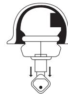
*Fig. 2) Insert the Allen supplied into the Allen socket – turning it to the right will spread out and fix the ball into place.*
